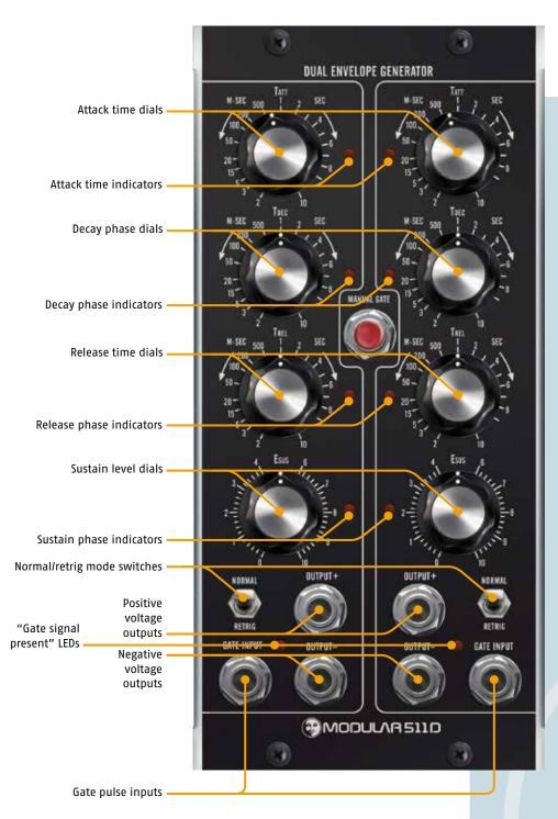
The 511 D **DUAL ENVELOPE GENERATOR** module in typical ADSR–Style with four parameters: attack time, decay time, release time and sustain level.
