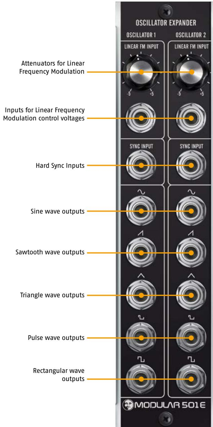
The M 501 E **OSCILLATOR EXPANDER** adds more inputs and outputs to the 501 D dual oscillator.
