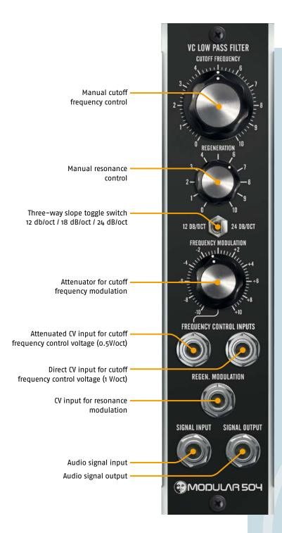
The M504 VOLTAGE CONTROLLED LOW PASS FILTER is a traditional ladder-type low pass filter, switchable 12/18/24 dB/oct slope with voltage controllable cutoff frequency and regeneration.
