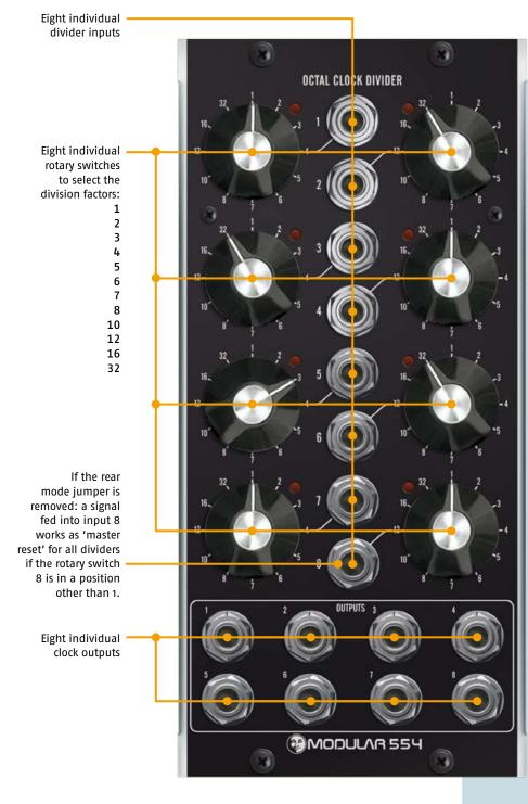
The M 554 **OCTAL CLOCK DIVIDER** combines eight divider circuits in one module.
