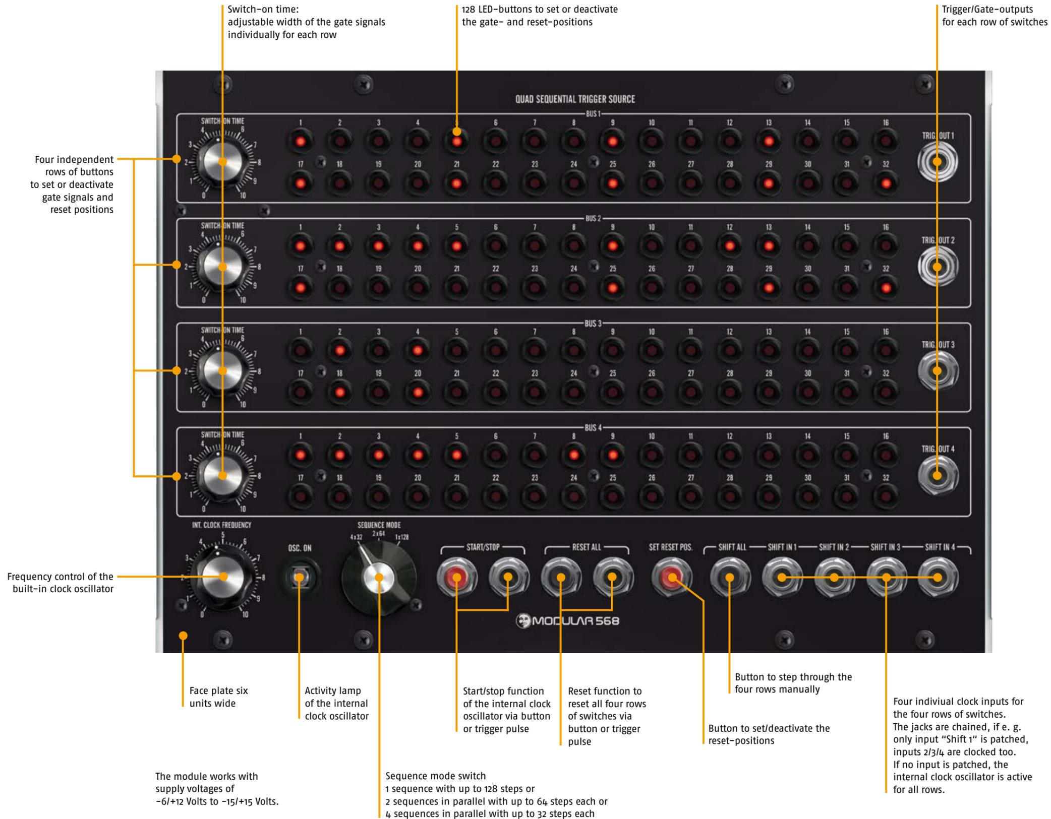
The M 568 **QUAD SEQUENTIAL TRIGGER SOURCE** is an elaborated trigger sequencer. It features four tracks of trigger positions, each with 32 steps, which can be combined to one long sequence of up to 128 steps:
