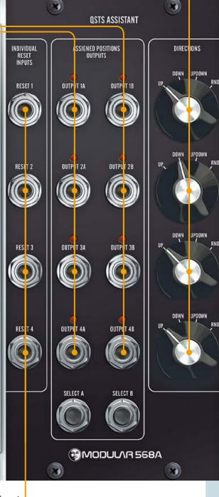
Four individual reset inputs for track 1–4 of the 568 QSTS
