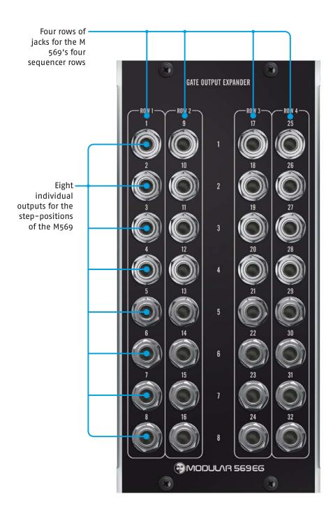
The M569 EG is a companion module to the M569 quad sequential voltage source.
